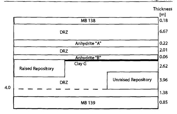
Figure 3. Schematic of the stratigraphy surrounding the raised and unraised sections of the repository. Not to scale.
